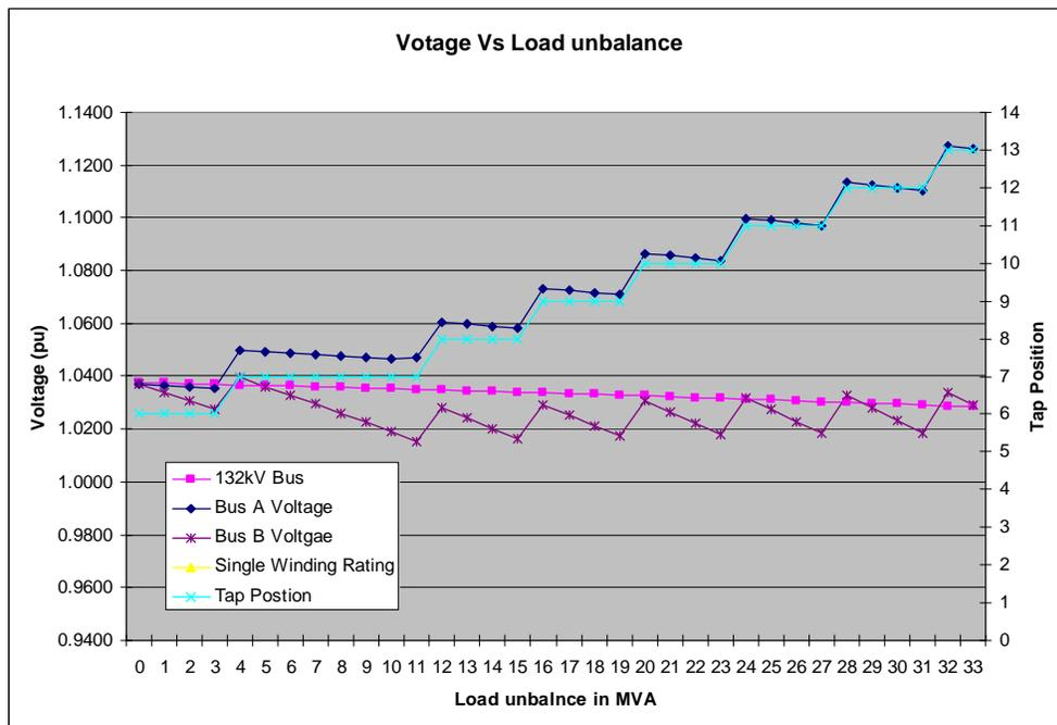
Figure 18: Load unbalance vs. Voltage (132kV)
