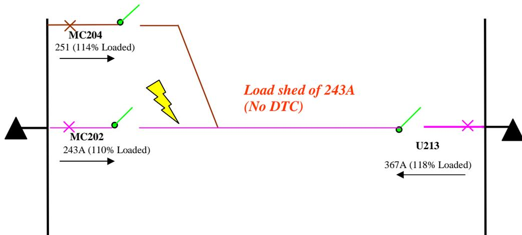
**Figure 10: Fault during summer 2014/15 peak loading (MC202 off-load scenario)**
