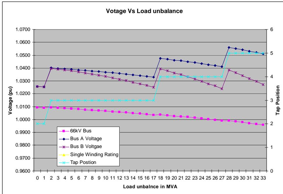
Figure 17: Load unbalance vs. Voltage (66kV)
