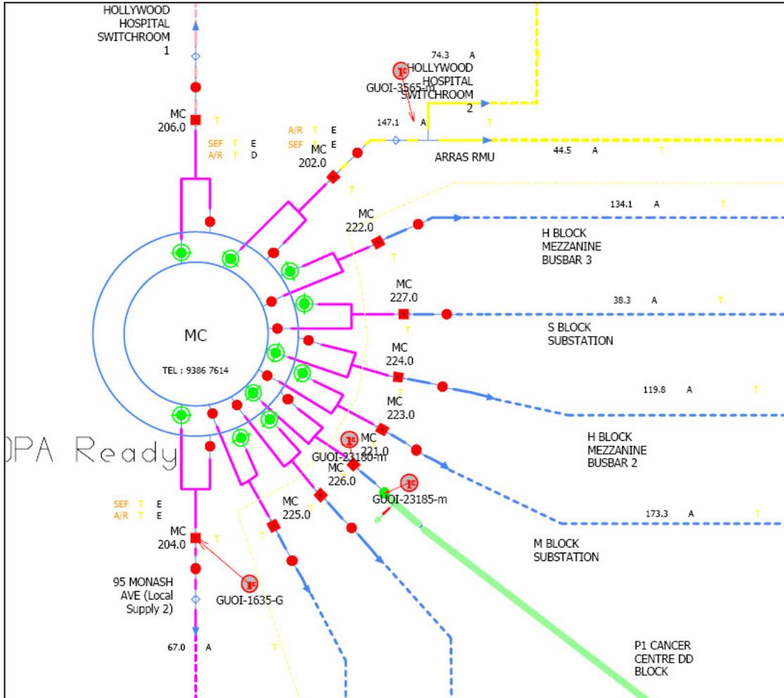
Figure 14: Medical Centre distribution feeder circuits
