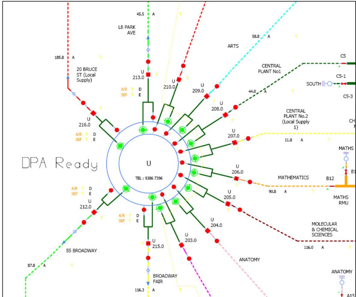
Figure 15: University distribution feeder circuits
