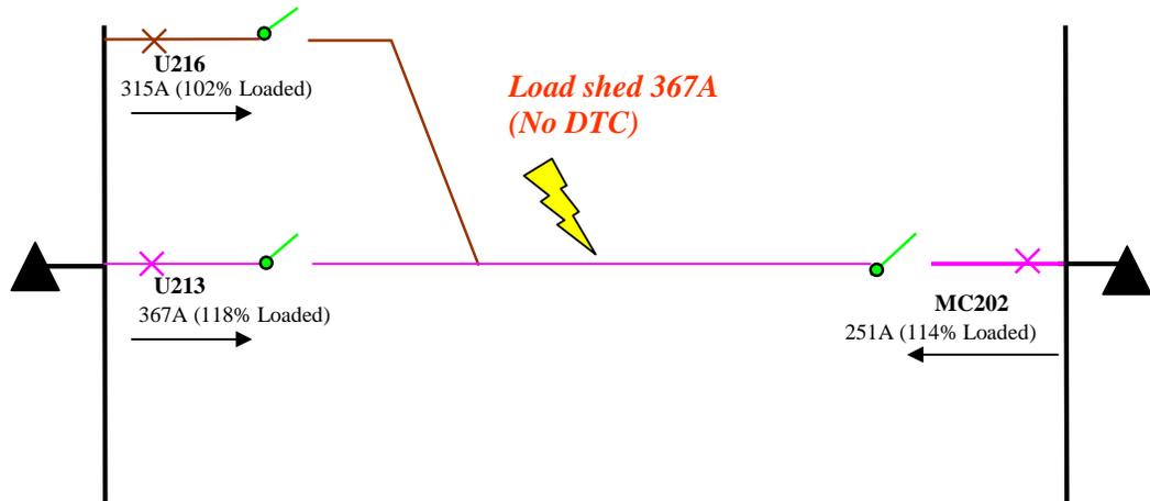
**Figure 11: Fault during summer 2014/15 peak loading (U213 off-load scenario)**
